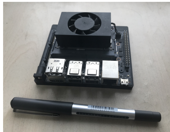
Fig. 1. Nvidia Jetson XAVIER NX. Mechanical 103 mm \times 90.5 mm \times 34.66 mm.
